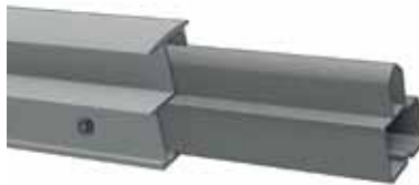
Shift one half of the connector into the purlin and fasten it with a self-drilling screw
