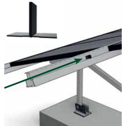
Join the bottom spacer to the inserted module
