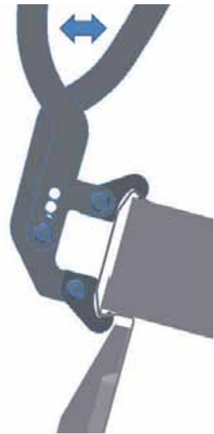
6 Release the clamp and take off the pliers
