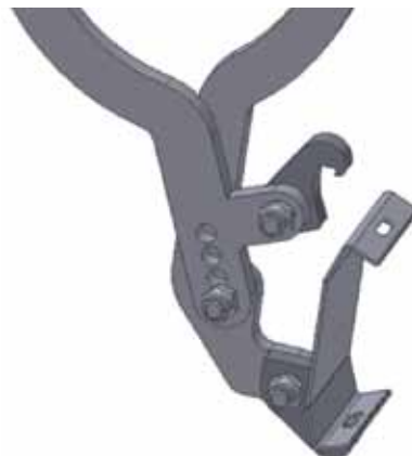
2 Put the clamp in the lower jaw
