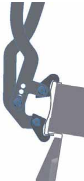
5 Put the clamp on the module and the AluGrid system.
