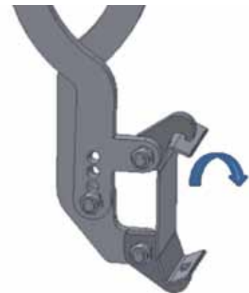
2 Put the clamp in the upper jaw
